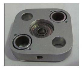
This part will be used in order to maintain the alignment when the shafts will be glued on the Motor Cap P/N: 002-400-P-1022
