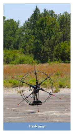
The HexRunner "demonstrated that high-gain feedback and actively controlled foot placement is not necessary for stable bipedal running," said IHMC Research Associate Johnny Godowski.
