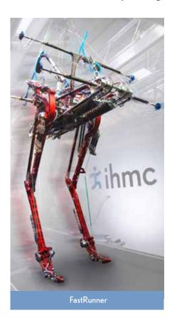
speeds of 40 mph. But on the treadmill, the actual robot, with its meter-long aluminum legs and powerful hydraulic actuators, slammed the ground with too much force and failed to achieve optimal running performance.
