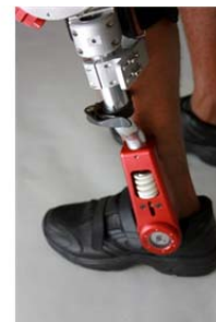
Figure 5: Original Mina ankle joint shown with spring. The joint is coincident with user's ankle joint and restricts rotation to dorsi/plantar flexion only. The neutral position of the spring is with five degrees of dorsiflexion. This flexible joint was replaced with a rigid joint that prevented movement of the ankle joint.
