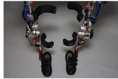
Figure 4: Placement of the C-shaped leg braces. The leg brace straps have been removed for clarity. Note that the thigh braces provide a rigid support at the back of the leg and the shank braces provide a rigid support at the front of the leg.
