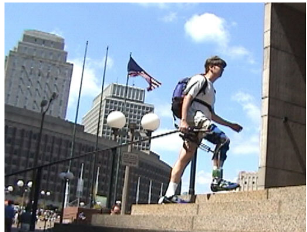
Figure 1. RoboKnee (on right leg only) providing power required to climb stairs at City Hall, Boston on August 24, 2001. The backpack contains the computer system and 4 kilograms of Nickel-Metal-Hydride batteries, enough to power the system for 30-60 minutes of heavy usage.
