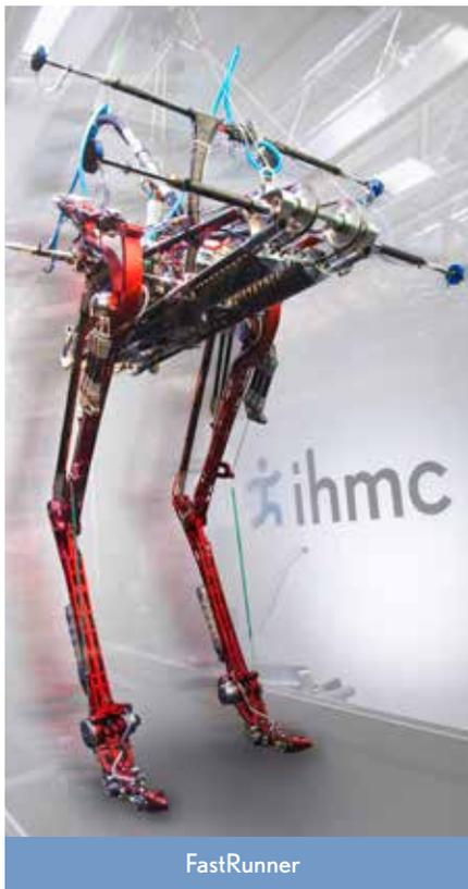
speeds of 40 mph. But on the treadmill, the actual robot, with its meter-long aluminum legs and powerful hydraulic actuators, slammed the ground with too much force and failed to achieve optimal running performance.
