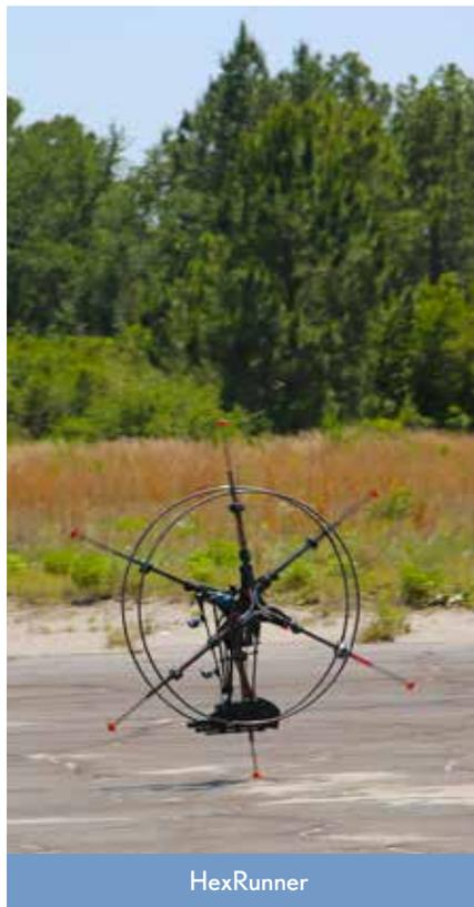
The HexRunner "demonstrated that high-gain feedback and actively controlled foot placement is not necessary for stable bipedal running," said IHMC Research Associate Johnny Godowski.
