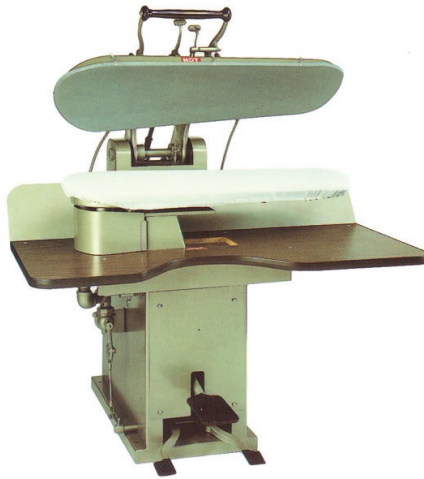
A Hoffman steam pressing machine similar to those I worked on.
