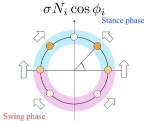
**Figure 2:** Schematic of oscillator dynamics depending on local sensory feedback  $\sigma N_i \cos \phi_i$ .
