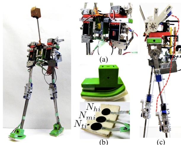
**Figure 1:** Constructed bipedal robot: (a) waist section, (b) soft foot, and (c) knee reflex mechanism.
