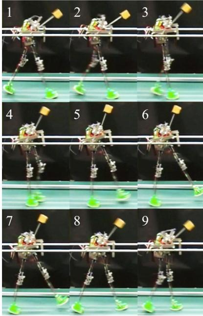
**Figure 4:** Photographs taken during steady walking at 0.10 s intervals.
