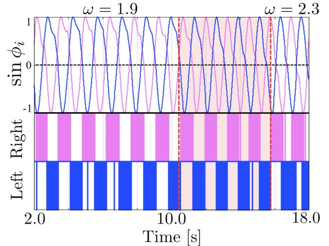
**Figure 5:** Experimental results of transition during a change in walking velocity by changing  $\omega$ .
