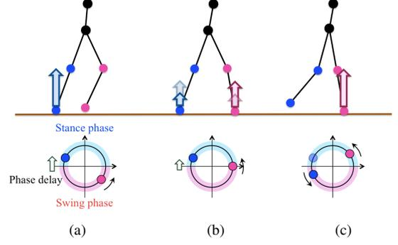
**Figure 3:** Schematic showing the physical effect of local sensory feedback. The pink and blue points in the lower part of the figure denote the phases  $\phi_i$  of the right and left legs oscillator, respectively.
