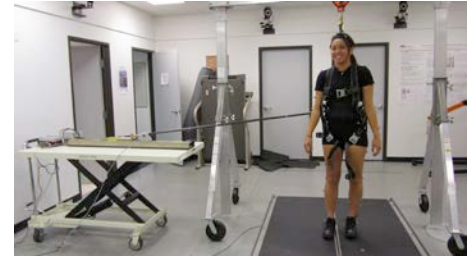
Figure 2. Device to directly perturb walking and running.
