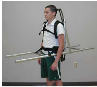
Figure 1. Device to increase moment of inertia ( I ) consisting of a backpack frame with two 1.4 m galvanized steel poles attached to the hip. Weights added to different locations on the increase M and I . The device weighs 5.7 kg.
