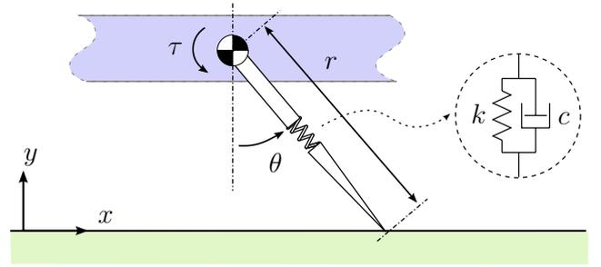
**Figure 1:** TD-SLIP : Planar, dissipative spring-mass hopper with rotary hip actuation [2]
