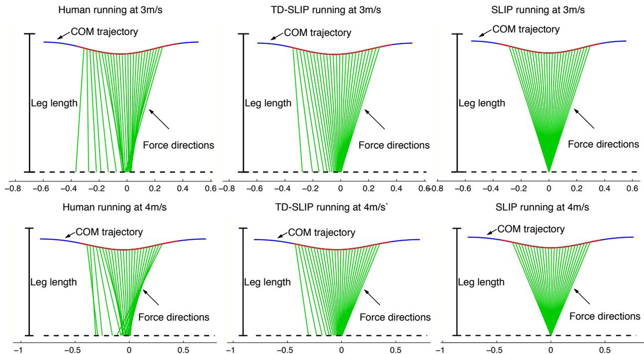
**Figure 2:** Center-of-mass trajectories and effective footprints of human, TD-SLIP and SLIP running at 3 m/s and 4 m/s. Green lines show the directions of GRFs as in [17].
