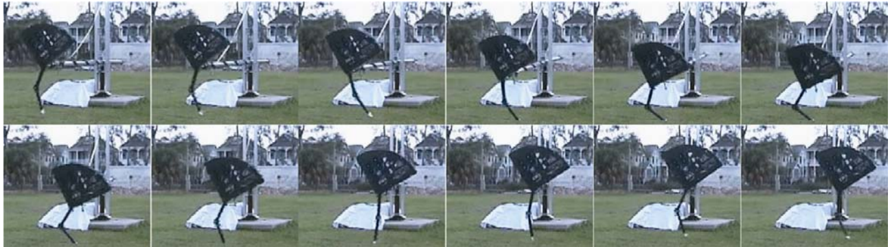
Figure 10: Monopod running with full component weight of approximately 125 pounds, but powered from off-board hydraulic source. Images are spaced at 0.1 seconds. Robot runs from left to right.
