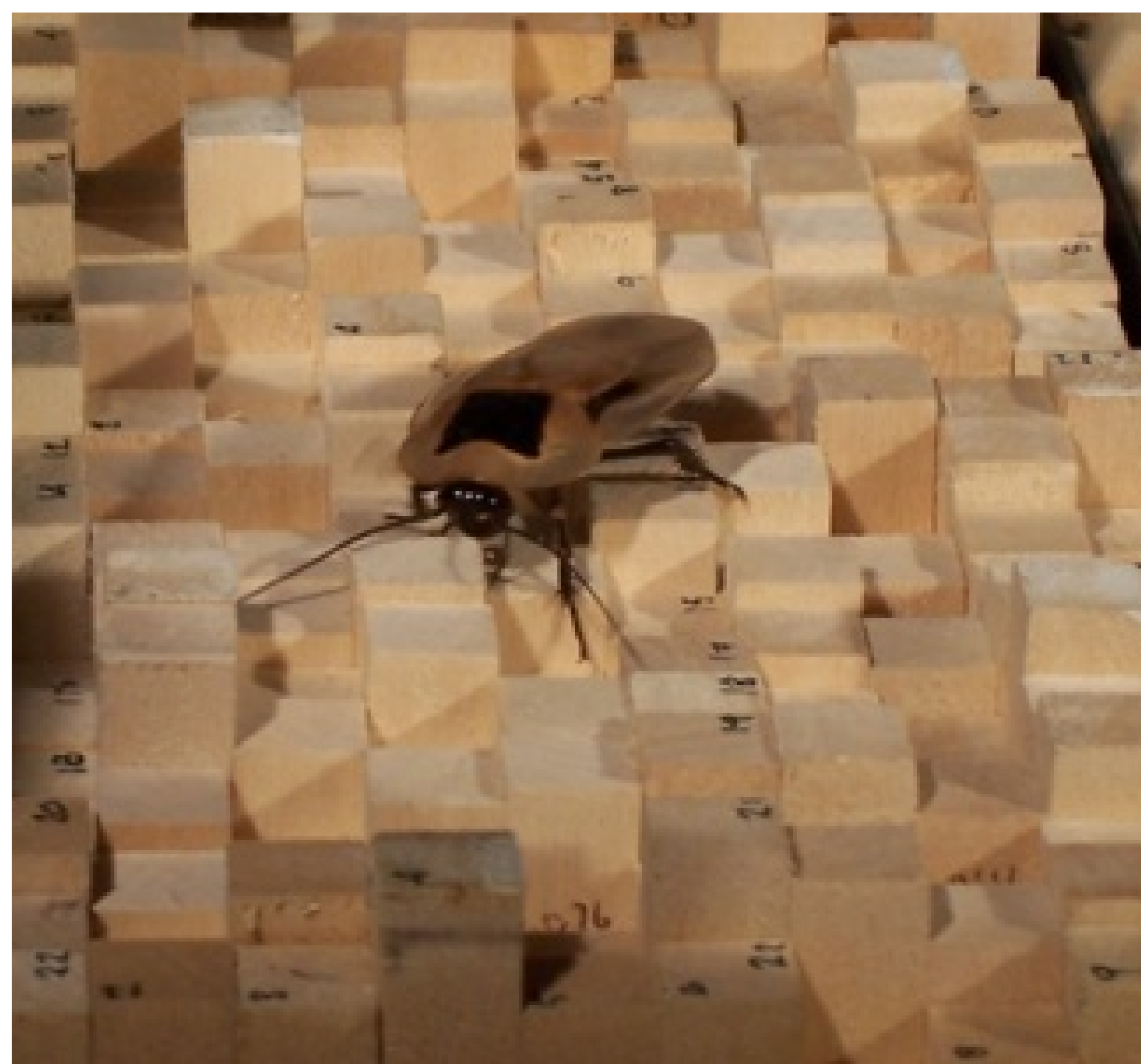
Figure 1: Blaberus discoidalis on rough terrain with a random distribution of surface heights.
